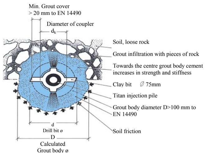
**The new reinforced tendon consist of a steel tube which is continuously threaded and composed of fine grain structural steel**
