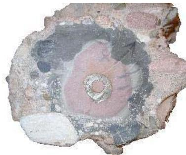
A longitudinal section of a grout body shows regular, fine cracks within the hardened cement paste, the cracks are directed away from the ribs of the tendon.
