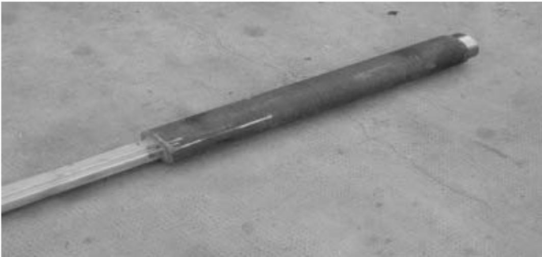
*Blocking system with Glasspree® flat bars system: Ultimate tensile strength 800 kN*
